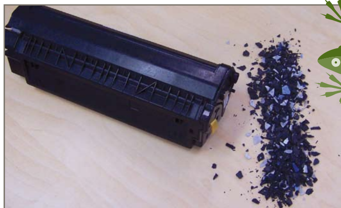
A remanufactured cartridge ready for reuse, and another at the end of its life, chipped and ready for recycling
